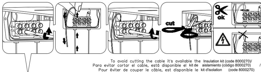
To avoid cutting the cable it's available the Insulation kit (code 8000270) /
